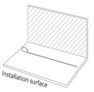
**Step 4** Install the adjustable clips with mounting channel by pushing them into the groove of the adjustable clips.
