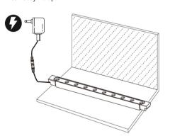
**Step 2** Determine the desired location and lengths of neon to be installed. Leave enough distance for power cable to reach the power supplies.
