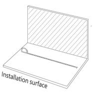
**Step 4** Install the adjustable clips with mounting clips by pushing them into the groove of the adjustable clips.
