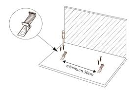
**Step 5** Gently push the neon into the mounting clips from one direction with palm instead of finger.
