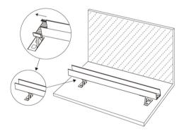
**Step 6** Plug in power after installation, make sure the neon flex is correctly lit up. Adjust to the adjustable clip to a desired angle.
