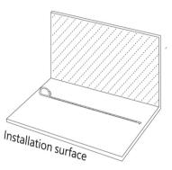
**Step 4** Gently push the neon into the channel at the beginning of the run with palm instead of fingers and moving down the line towards the end.
