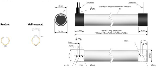
4 Standard lengths (L): 800 mm / 1,050 mm / 1,300 mm / 1,550 mm
