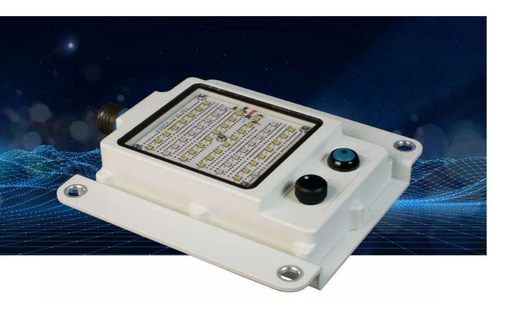
This series is new generation dome lights having a high light intensity and special operational features. With a low profile design, it is a perfect solution for illuminating land vehicles, vessel and mobile tactical shelters. Two operation modes are available, White light mode and Blackout light mode, selectable by a pushbutton. Light intensity is controllable from 5% to 100%.
