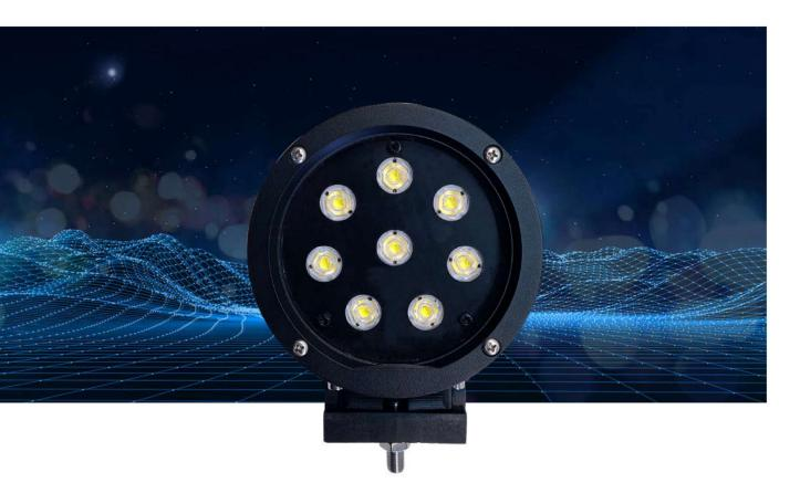
The LED based head light is designed to provide wide angle illumination for armored vehicles. The design utilizes a solid-state constant current drive circuit to achieve a consistent and efficient light output at an input voltage range of 16-33VDC.
