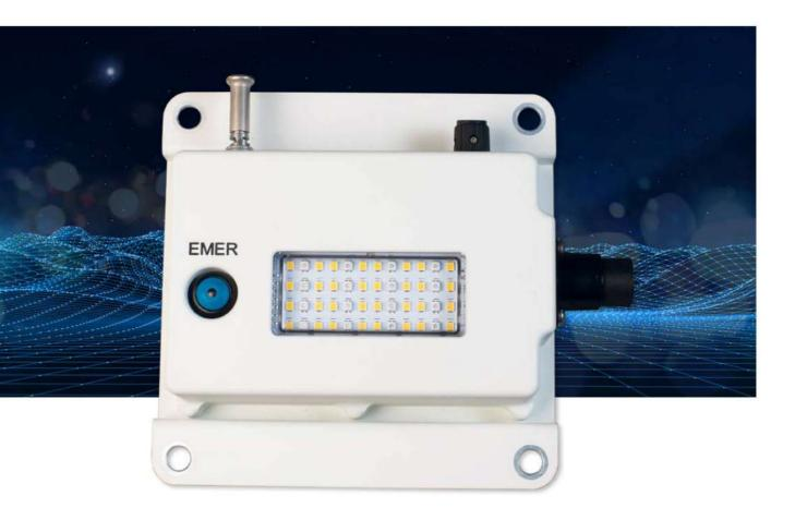
The LED based dome light is designed to provide general purpose illumination within armored vehicles. Two operation modes are available, White light mode and Blackout light mode, selectable by a 3-state toggle switch with a lockout lever.
